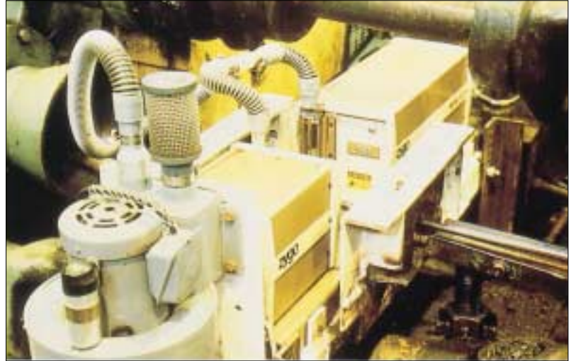
Bottom: Tensile testing at up to 1200°C (2190°F).
