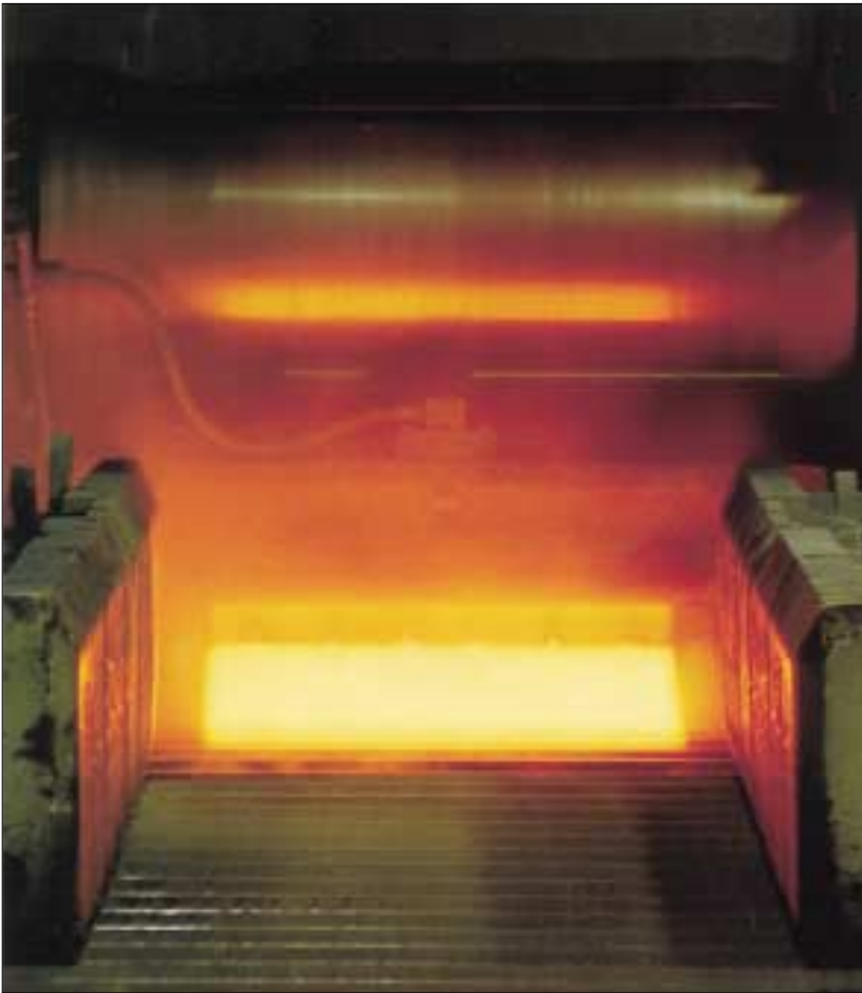
Left: Hot rolling at Special Metals Corporation, Huntington, to produce plate products 4.7 to 150 mm (0.2 to 5.9 in) thick, up to 2591 mm (102 in) wide.
