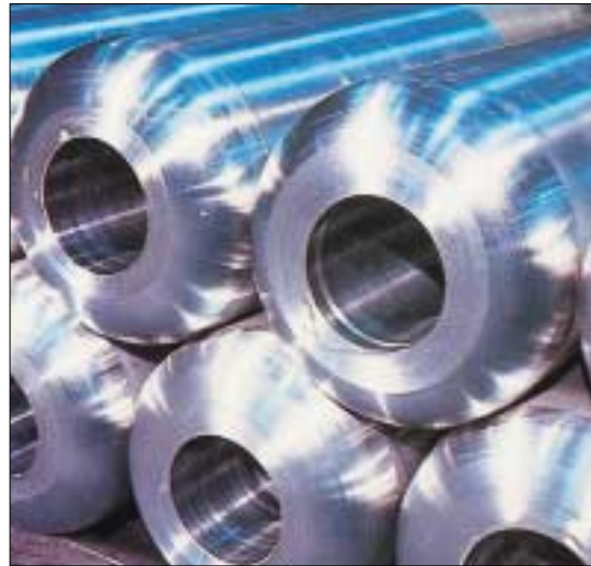
Below: Trepanned billets ready for extrusion at Special Metals Corporation, Burnaugh, Kentucky.
