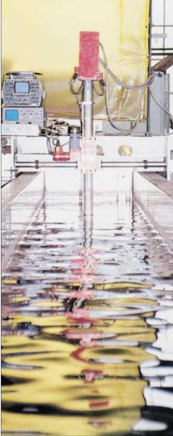
Left: Ultrasonic testing of tubular products.
